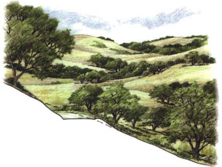
Grading standards require blending cut and fill slopes into surrounding landforms.
